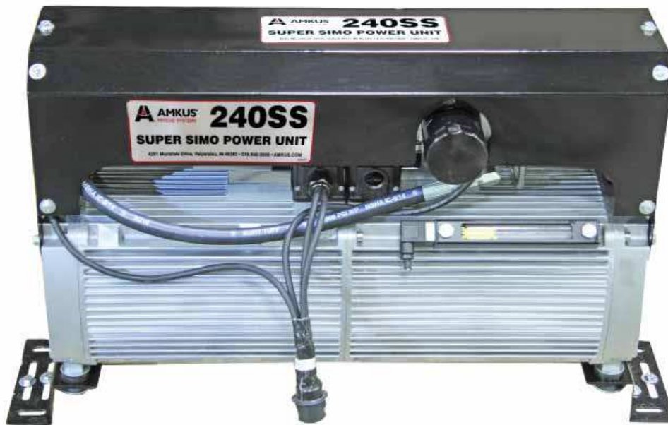
Electrically driven, truck mounted, 10,500 PSI (720 bar) twin pump hydraulic power unit for simultaneous operation of two rescue tools.
